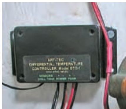
A DC-powered differential controller, designed and built by the author.
